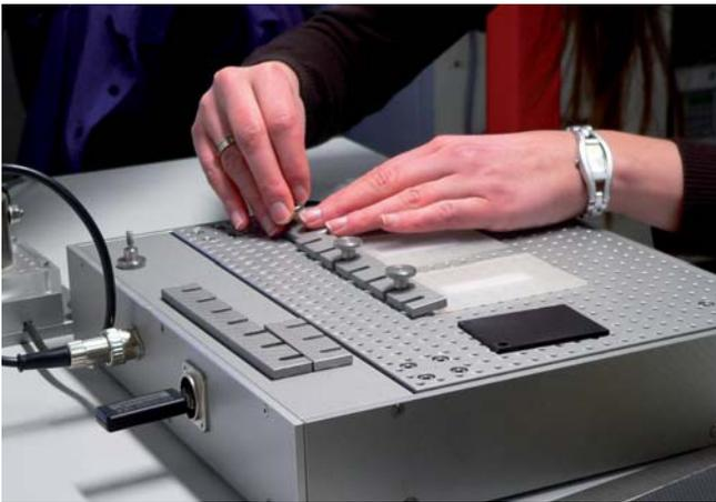
*The different materials are mounted on the force measurement plate for analysis.*
